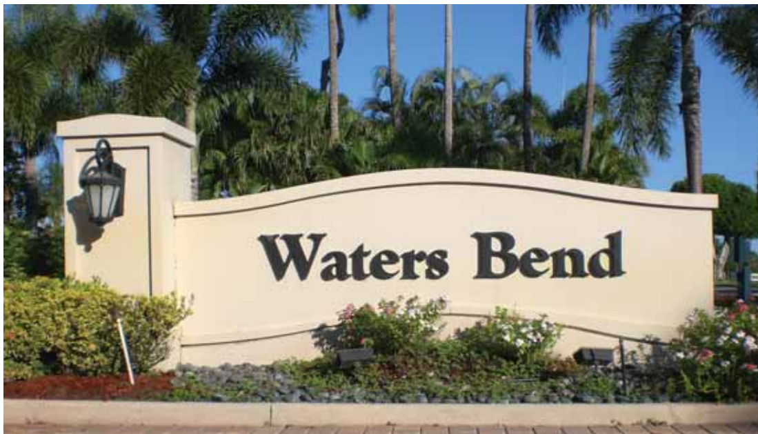
5½-by-16½-ft. double-faced HDU sign with copy cut from HDU board
