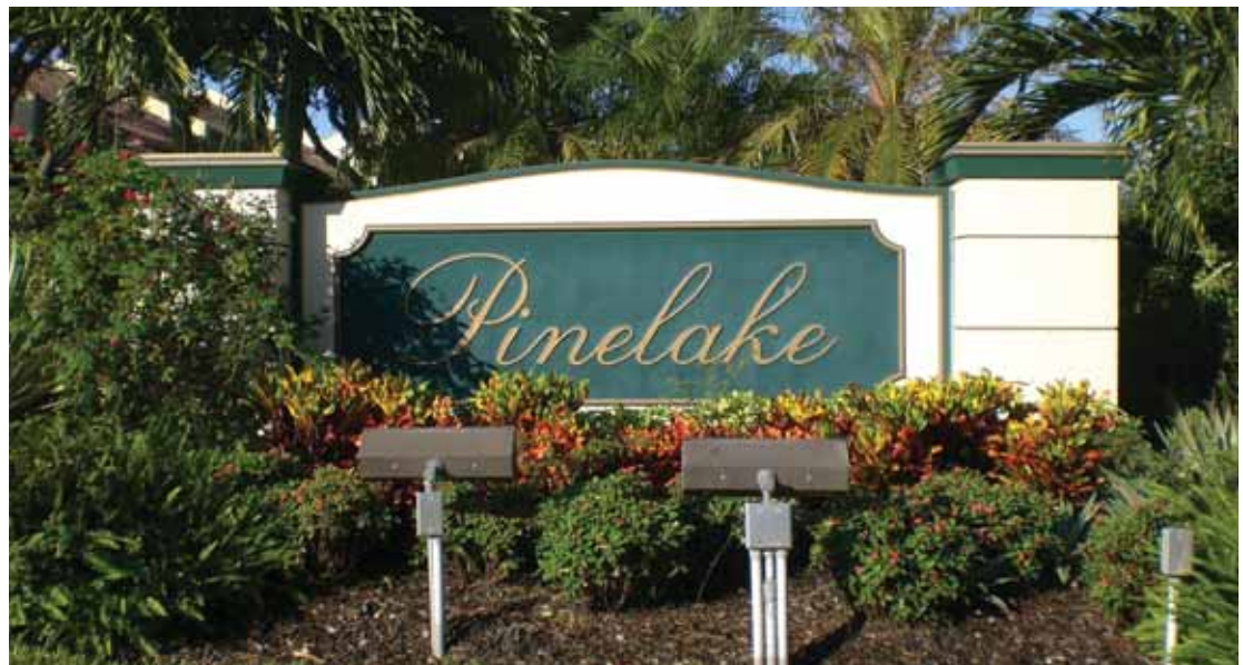
5-by-10 \frac{1}{2} -ft. sign of Sign•Foam high-density urethane board [Sign•Arts Products, 800-3384030, www.signfoam.com ] laminated to overlaid plywood; with a simulated stucco finish and a sandblasted sign face
