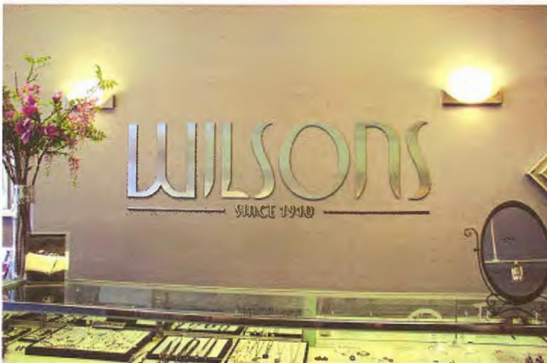
*These letters are for interior and exterior use. They are precision cut from .032 inch metal laminated to an acrylic backing.*
